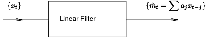
Figure 1-20 Smoothing with a low-pass linear filter.
